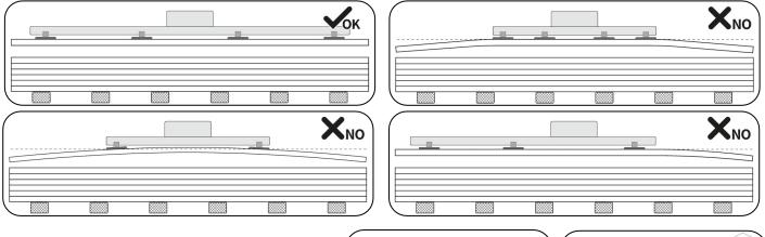
The following are, by way of example, two conceptual solutions for correct suction cup systems in which the suction cups are properly distributed according to the length of the panel.
