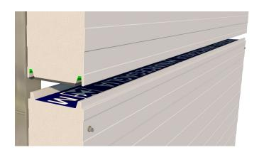
Fix the second panel to the structural uprights with the appropriate screws in one of the two ways shown in the images below.
