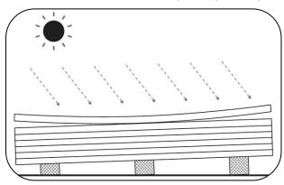
In order to maintain the original performance of the product, it is advisable, in accordance with these standards, not to exceed six months of continuous storage in a closed and ventilated environment, while storage in the open air should never exceed two weeks. The materials must always be protected from direct sunlight, as this can cause deterioration. During assembly, panels subjected to sunlight suffer a bowing that makes assembly difficult, so it is recommended to shade the parcel in use.
