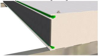
Proceed with the installation taking care to verify the perfect uprightness of the panel using temporary clamps or pliers.
