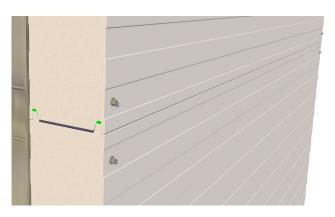
Similarly, proceed with the installation of the subsequent panels to the top of the wall.
