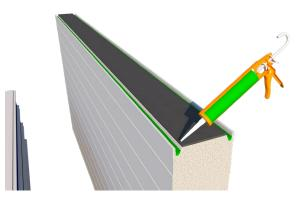
After horizontal installation of the base flashing on the structure, identify the starting point for the installation of the first panel on the working drawings.
