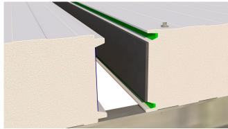
Check to ensure the parts are correctly mated and proceed with securing the panel as shown in the image below.
