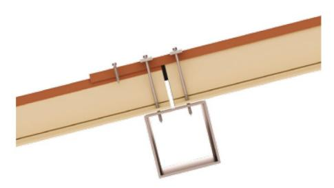
In this way shear stresses are more effectively discharged on the supporting structure, through fixing units. This layout is suitable above all for overlapping panels of great length.
