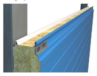
Check that the panel is perfectly horizontal and fasten it with through screws to the structural uprights along both ends of the panel and then near the male joint by placing a steel distribution plate between the screws and the panel. Screws must be of appropriate length (see section on vertical installation).
