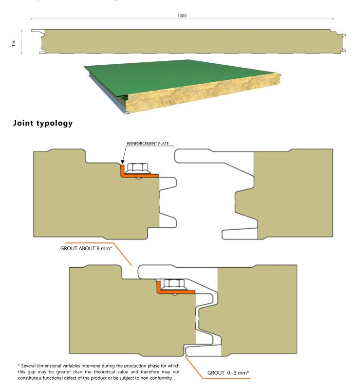
Thanks to its shape, the concealed fixing joint designed by Marcegaglia RWD allows the creation of walls that permit concealed fixing systems while still guaranteeing the functionality of the product.
