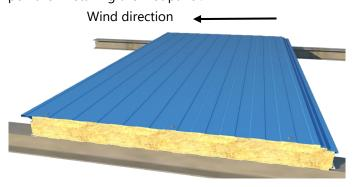
Fasten the panel along both ends to the steelwork on the rear with through-head screws and then the male joint, placing a steel reinforcing plate between the screws and the panel.
