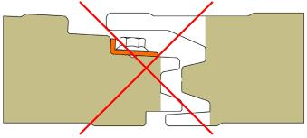
Pay close attention to the correct tightening of the screws, as over-tightening may deform the joint and cause imperfections.
