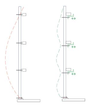
If the panel were fastened at the ends only, a curvature due to thermal expansions, such as the one shown in red in the figure, would occur. Normally, fastening systems provided for the panels lead to a curvature similar to that shown in green.
