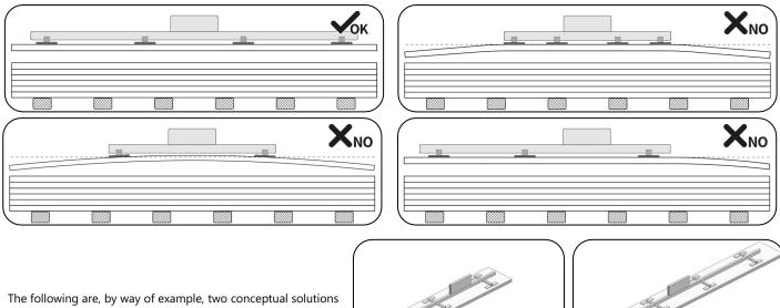
for correct suction cup systems in which the suction cups are properly distributed according to the length of the panel.
