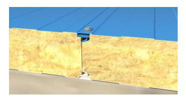
Proceed in similar fashion with the installation of the subsequent panels to the end of the wall.
