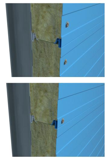
Similarly, proceed with the installation of the subsequent panels to the top of the wall.
