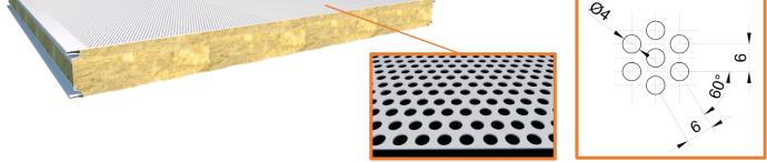
To increase the acoustic properties, the metal support on the inner side of panels is perforated with 4 mm diameter holes (R4T6), arranged in a triangle with centre distances of 6 mm, to generate an intermittent arrangement.
