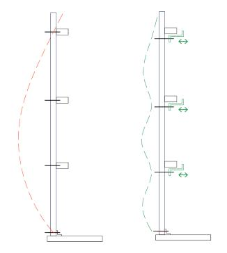
If the panel were fastened at the ends only, a curvature due to thermal expansions, such as the one shown in red in the figure, would occur. Normally, fastening systems provided for the panels lead to a curvature similar to that shown in green.
