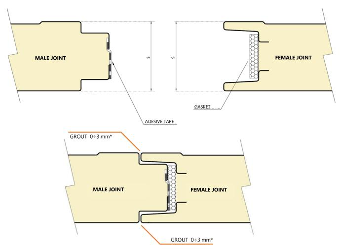
$\ensuremath{^{\star}}$  Several dimensional variables intervene during the production phase for which this gap may be greater than the theoretical value and therefore may not constitute a functional defect of the product or be subject to non-conformity.
