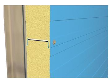
Similarly, proceed with the installation of subsequent panels to the top of the wall.
